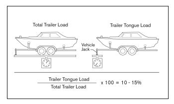
rearward of the trailer tongue and will not give you an accurate measurement of the true tongue load. Make sure the vehicle jack is placed directly under the trailer tongue coupler, and the tongue is set at the height/level of the tow vehicle hitch.
