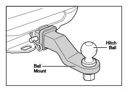
hitch ball in a 2" coupler, for example, could result in the trailer separating from the tow vehicle. The required hitch ball size is stamped on most trailer couplers.
