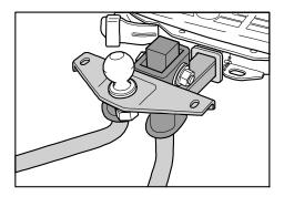
maximum weight over 5,000 lbs. This ball mount includes a 2-5/16" hitch ball and is available through your INFINITI retailer. Refer to trailer and hitch manufacturer for detailed information on load limits. Weight distributing hitches are available in many styles and with sway control accessory options to accommodate trailers with maximum loaded weight and for different driving conditions.
